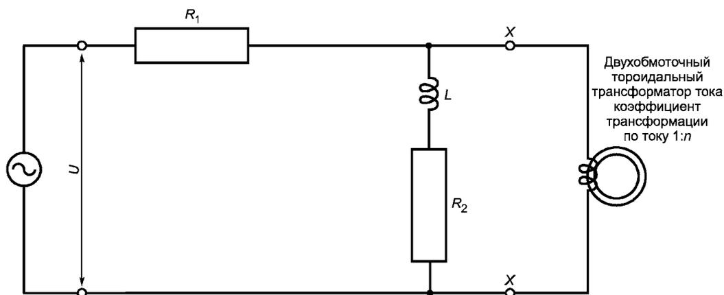
$$L = 80 n^2 \text{ мкГн } R_2 = n^2/4 \text{ Ом}$$
